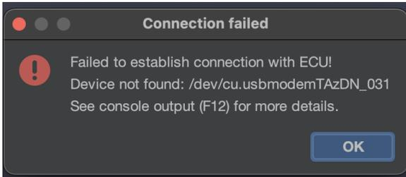
Sometimes, the OpenPort 2.0 can lose sync with the computer running Atlas. Make sure you always first connect the adapter to your computer running Atlas. Then, connect the OBD2 end of the Tactrix to the vehicle's OBD2 port, often located underneath the trim in the steering wheel area. Doing this in the reverse order can sometimes cause the Tactrix to incorrectly synchronize with your computer and Atlas.
